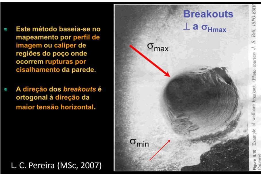
A **breakout** is the evidence of **wall yield** (the formation strength at the borehole wall is exceeded). A breakout **is not considered to be a borehole failure** since the borehole remains useful. Borehole breakout can be **measured** using four- or six-arm **caliper tools**. The preferred tool, however, is the **ultrasonic imaging tool**, which makes up to 200-caliper measurements at every depth level.
