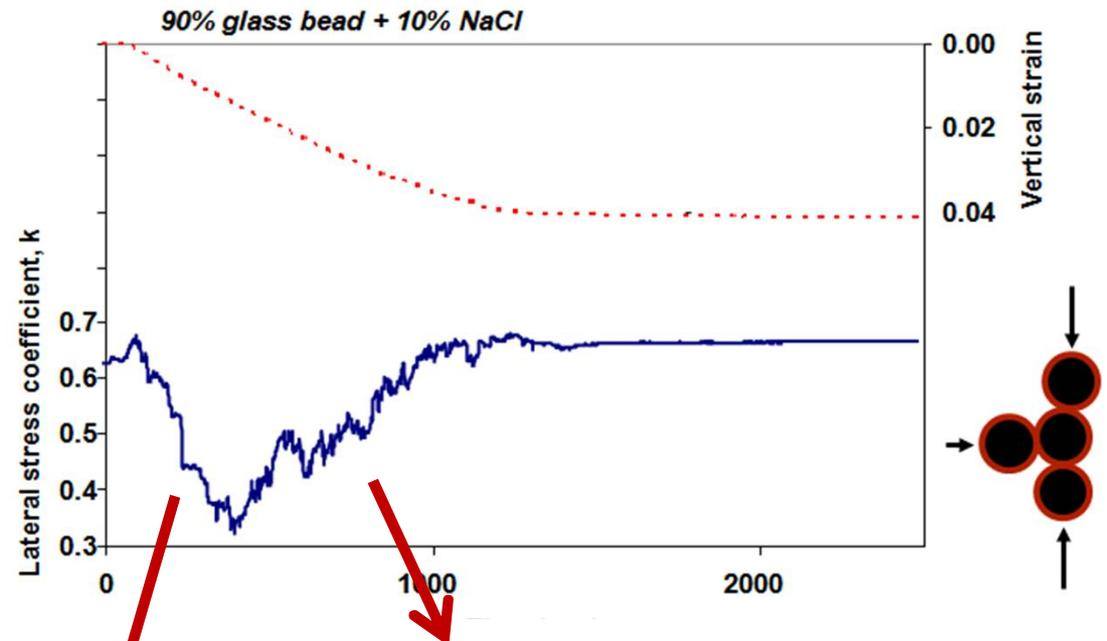
grain mass loss due to mineral dissolution produces a pronounced horizontal stress drop under zero lateral strain conditions
